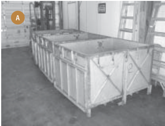
Figure 2. Steam boxes (A) with perforated floor (B) used for filling (C) and aerated-steam pasteurization (D) of Pleurotus spp. mushroom substrate.
