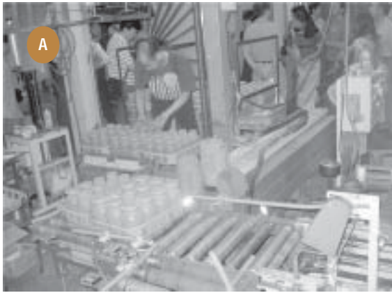
Figure 6. Process used for bottle production of Pleurotus eryngii . Bottles are filled and capped (A), autoclaved (B), the substrate is inoculated and incubated (C), and mushrooms are induced to fruit (D).
