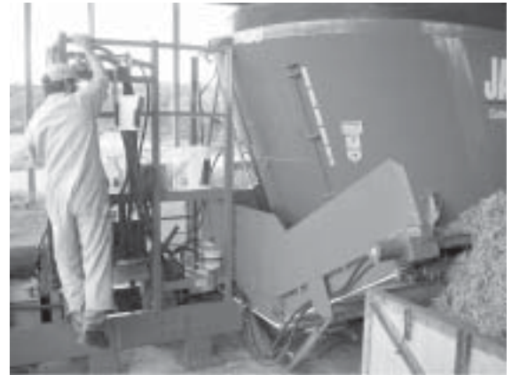
Figure 1. A large-capacity, scale-mounted feed mixer is used at the Mushroom Research Center (MRC) to process Pleurotus spp. mushroom substrates for filling into pasteurization containers.
